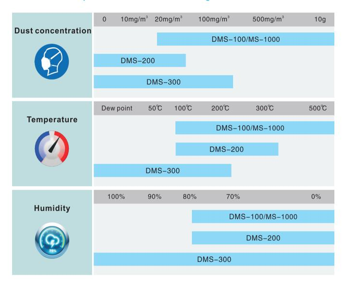
DMS Series Dust Monitor can be applied in power plant, cement plant, metallurgical and wood industry, chemical plant, waste incineration plant and etc.
